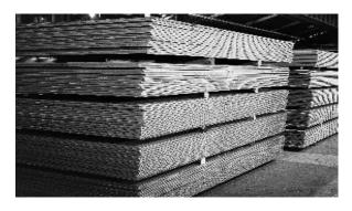
**Hot-rolled plates** are manufactured in a wide range of sizes for applications in several industries varying from construction to pressure vessels and wear-resistant chemistries.
